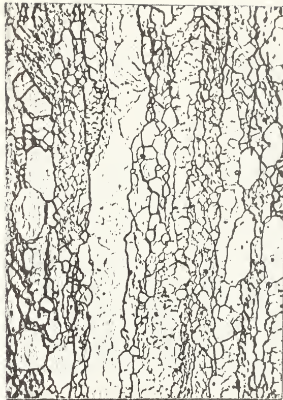
FIG. 34 AT 482°C, UNDER .6%/HR. STRAIN RATE, FOR 49 HOURS (ROCKWELL 30T 45.4)
